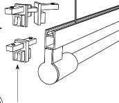
STJR-creates a mechanical connection for continuous runs. One connector is included with each two connecting fixtures.
